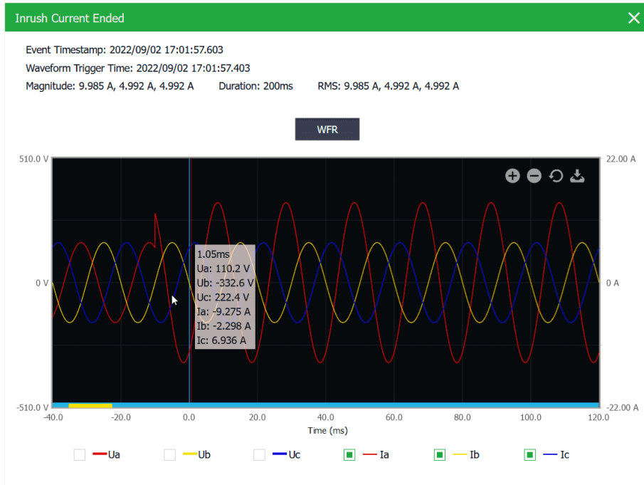
Figure 4-16 Inrush Current - displayed on Web Server
