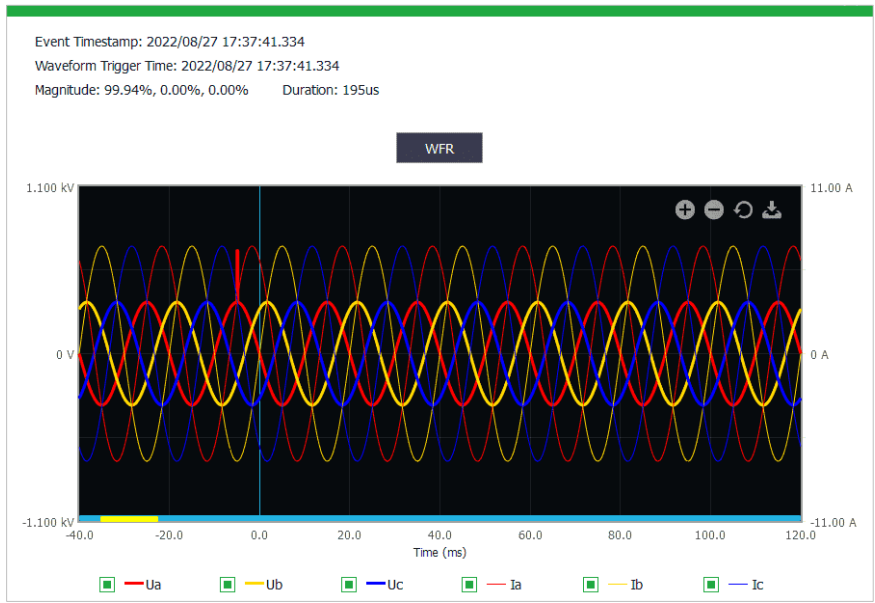
Figure 4-9 Transient Event @ 512 samples/cycle x 100 cycles
